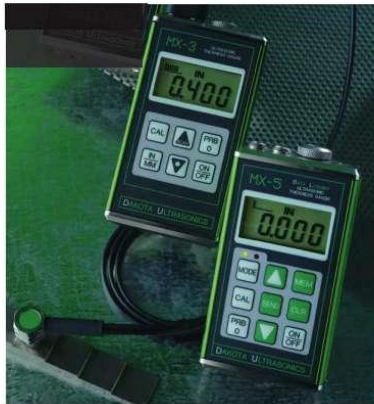
Fig. 2-2: Dakota MX-3 Ultrasonic Thickness Gauge made in USA
