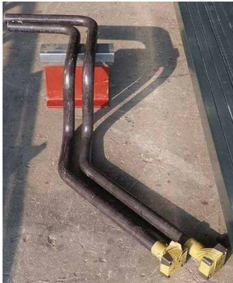
Fig. 2-1: 1.25" sch.160 (thickness 6.4t) hydraulic line (continuous 4 bends), ISO piping diagram
